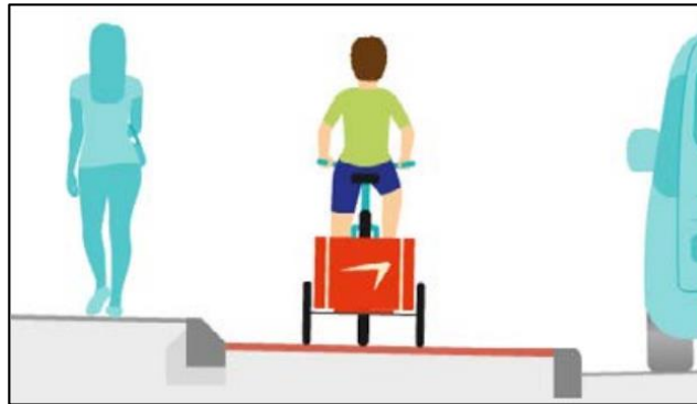
Figure 3-3 - Layout of stepped cycle track adjacent to carriageway (Cycling by Design, Transport Scotland 2021)
