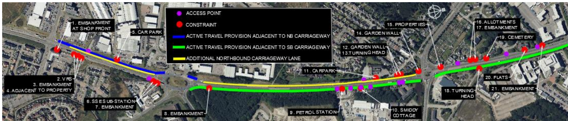
Figure 3-9 - Segregated Two-Way Flow Option with Bus Lane Constraints (©2023 Microsoft Corporation ©Maxar ©CNES(2023) Distribution Airbus DS)
